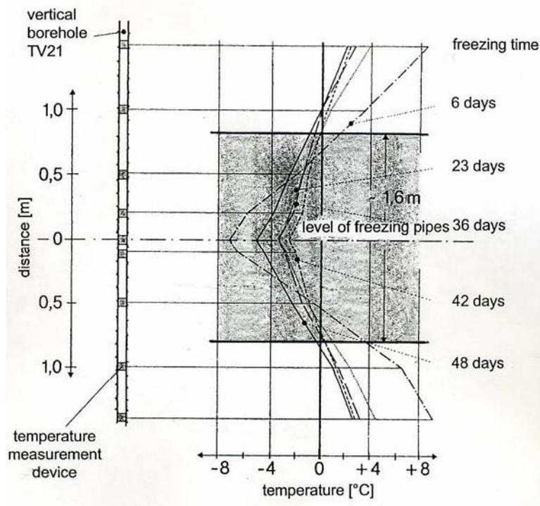
Fig. 3: Temperature distribution inside of frozen body (after Arz et al., 1988)
