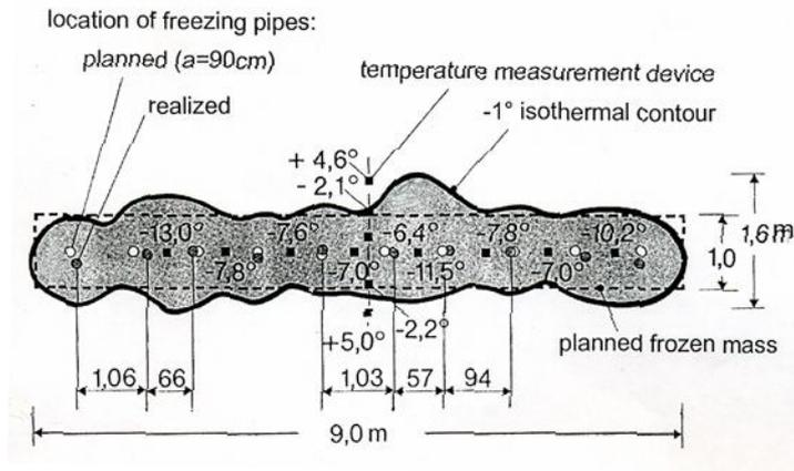
Fig. 4: Cross section of frozen body; 30 m far from shaft (after Arz et al., 1988)
