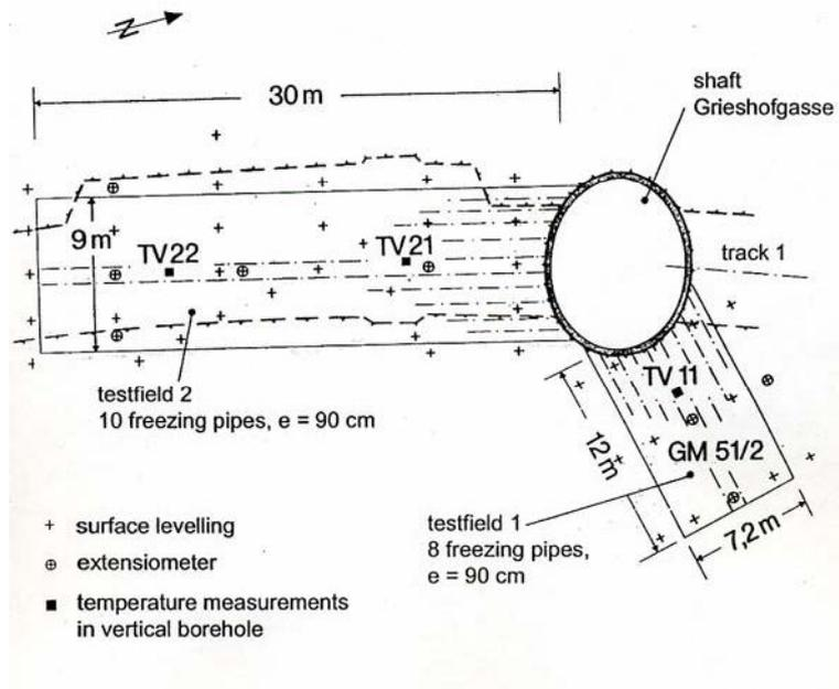
Fig. 2: Layout of test fields, construction lot U 6/3, subway Vienna (after Arz et al., 1988)
