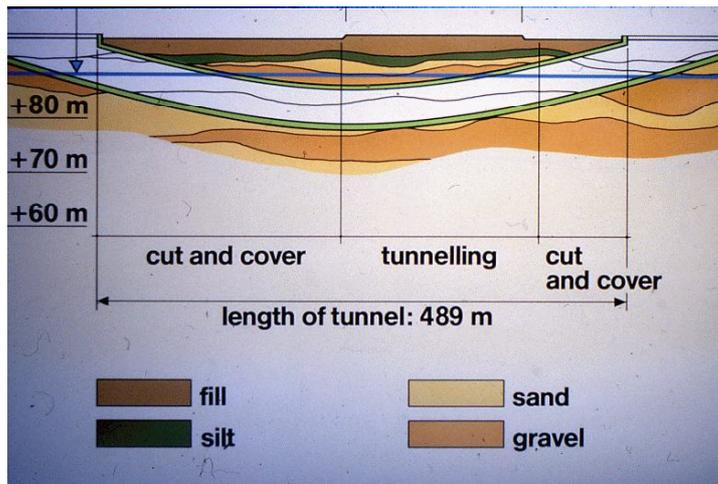
Fig. 6: Longitudinal section, Fahrlach Tunnel, Mannheim
