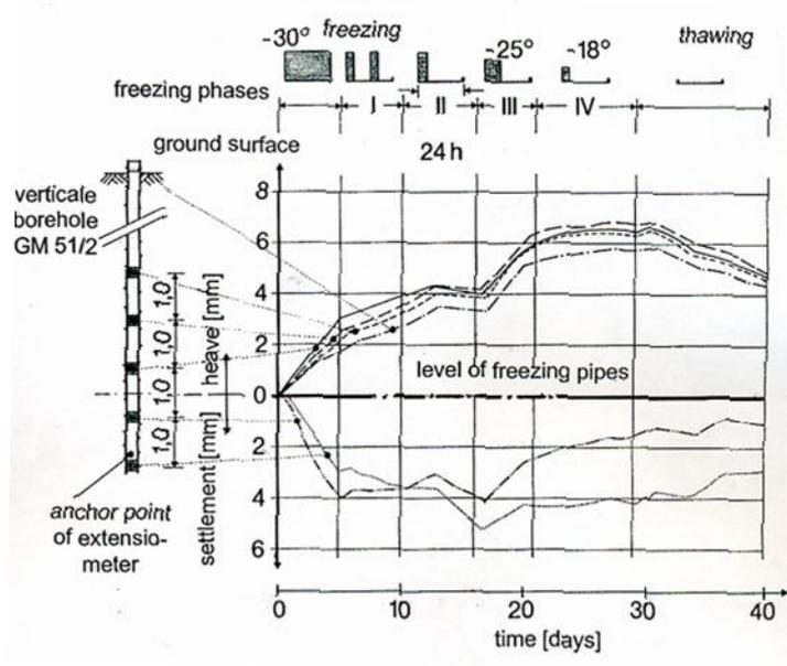
Fig. 5: Displacements of frozen soil along borehole GM 51/2 (after Arz et al., 1988)
